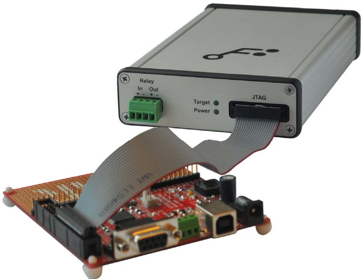
Illustration 6: Connecting the ZY1000 to your target.
