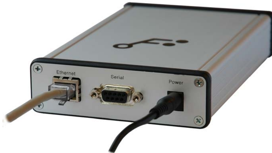
Illustration 3: ZY1000 Ethernet Connection.
